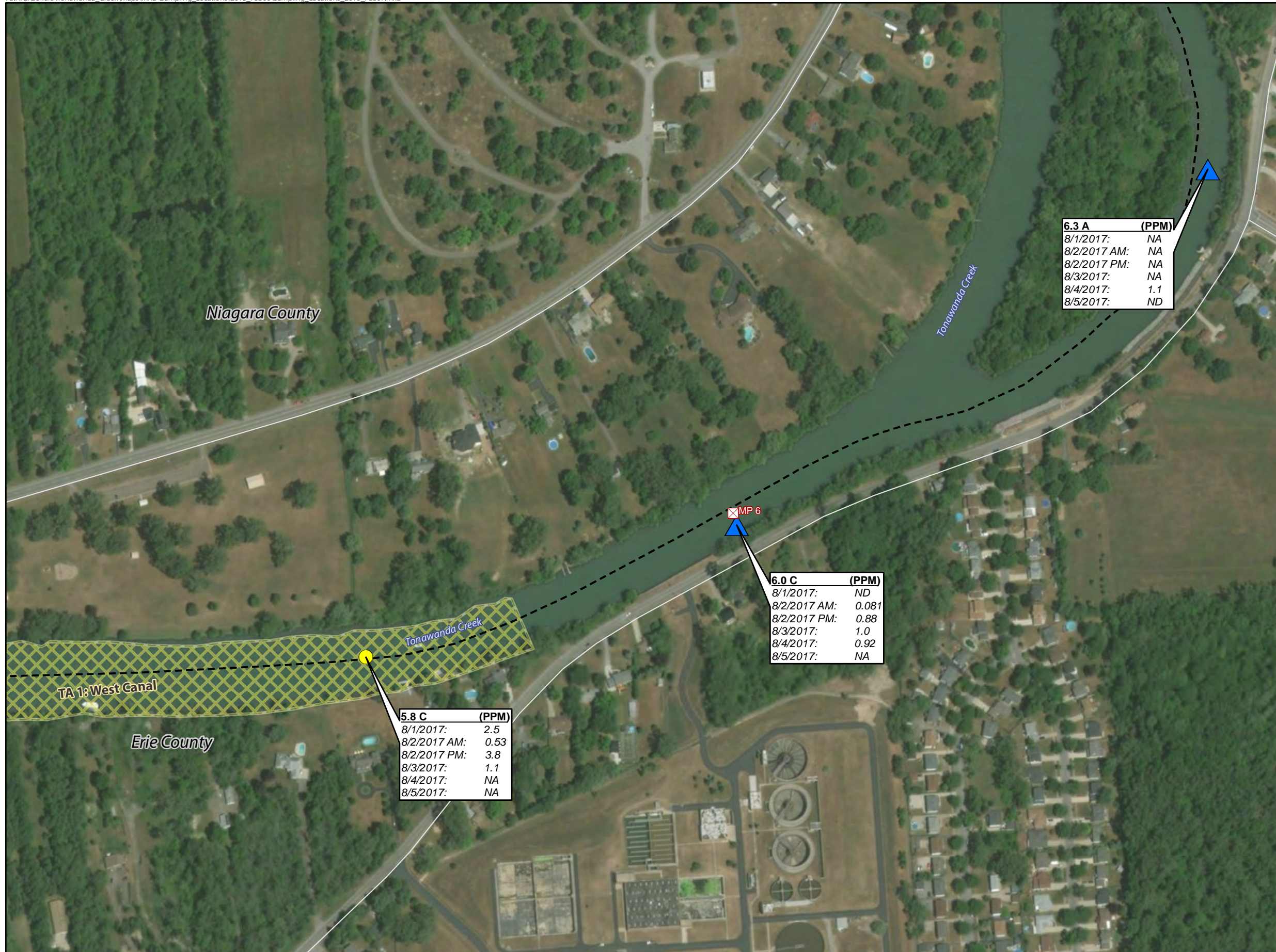
Sample Locations Associated Endothall Concentration Values Figure B9 Tonawanda Creek/Erie Canal Erie and Niagara Counties, New York
