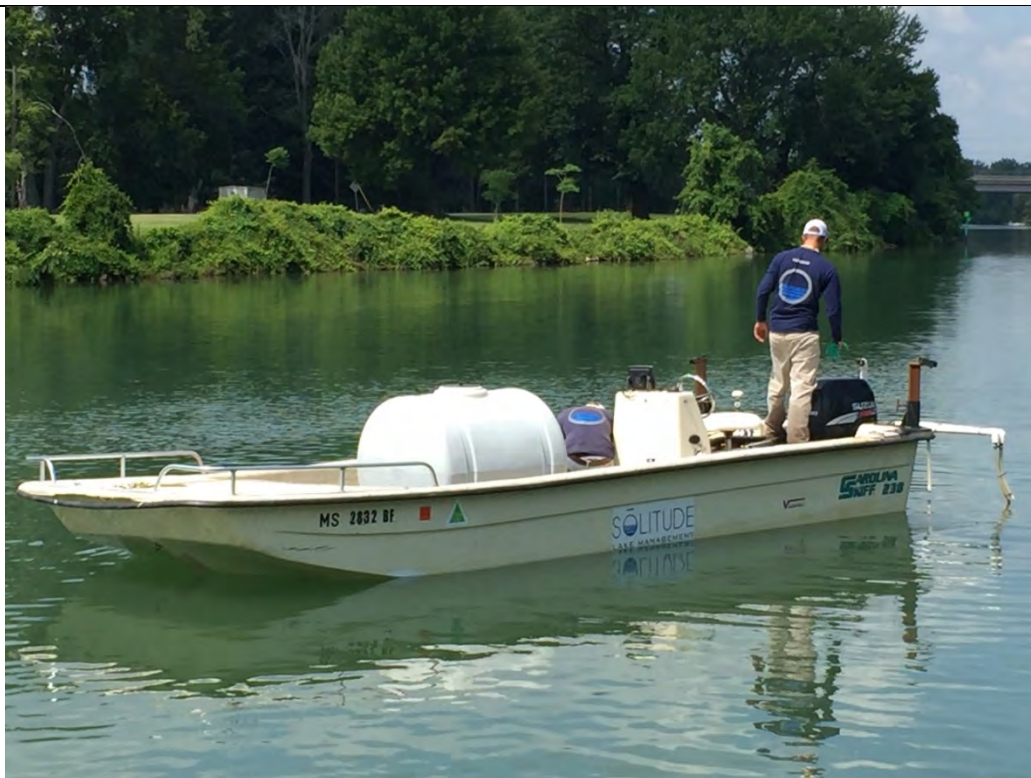
Date: 08/01/2017 Direction of View: West from North shore of creek Subject: SOLitude endothall application boat Description: Endothall was placed in the tank and dispensed into the creek/canal through PVC pipes off of boat stern.
